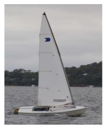
'You will note from the photos that they have had to use a full length batten in the top of the sail during these early stages in order to get the sail to set. Technically this does not fall within the class rules. They are looking at ways to overcome the need for the full length batten.
